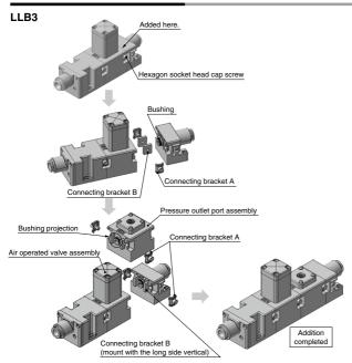
Example: Addition of the pressure outlet port assembly (LVB3-2)
