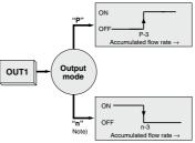
Note) Output mode is set to inverted output when shipped from factory.
