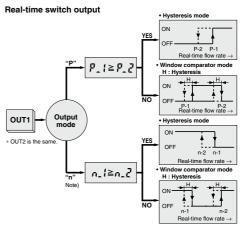
Note) Output mode is set to inverted output when shipped from factory.
